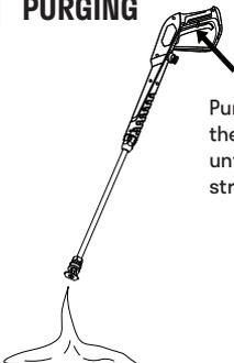
Purge air by squeezing the trigger on the gun until there is a steady stream of water.
